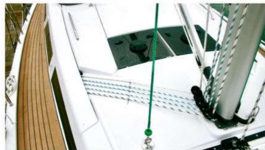
ABOVE Neat GRP mouldings cover the halyards, reef lines and sheets on their way to clutches on the cockpit coamings and self-tailing Lewmar 40 winches
