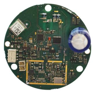
Figure 5: rescueME EPIRB PCB – Rear side with screening can removed.
