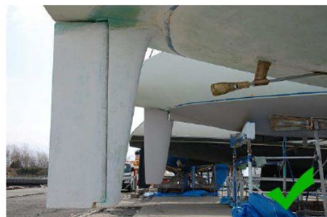
Skeg clearly visible as is propeller
