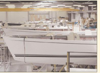
Hull and deck of the HANSE 312 are laminated in hand-laid sandwich construction and are firmly bonded together with a stable outside rail and high-strength glue. In the gel coat and in the outer laminate layers, high-quality isophthalic resin is used as an osmosis protection. The forces of rig and keel are absorbed by a strong floor segment.
