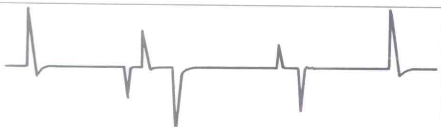
Fig. 15: the sort of waveform expected across the pickup coils. The amplitude and polarity of the pulses changes with strength and direction of the static magnetic field.
