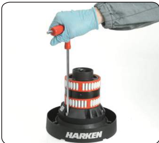
8. Unscrew the 5 hex screws n°17 ( \approx 20\text{Nm}/177\text{ in-lb} )
