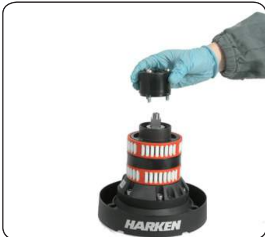
6. Completely unscrew the three screws n° 28 and remove the stripper arm support n°22
