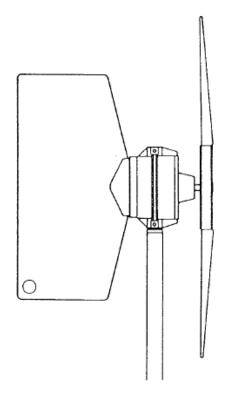
Figure 3. Wind Mode Pole Mount
