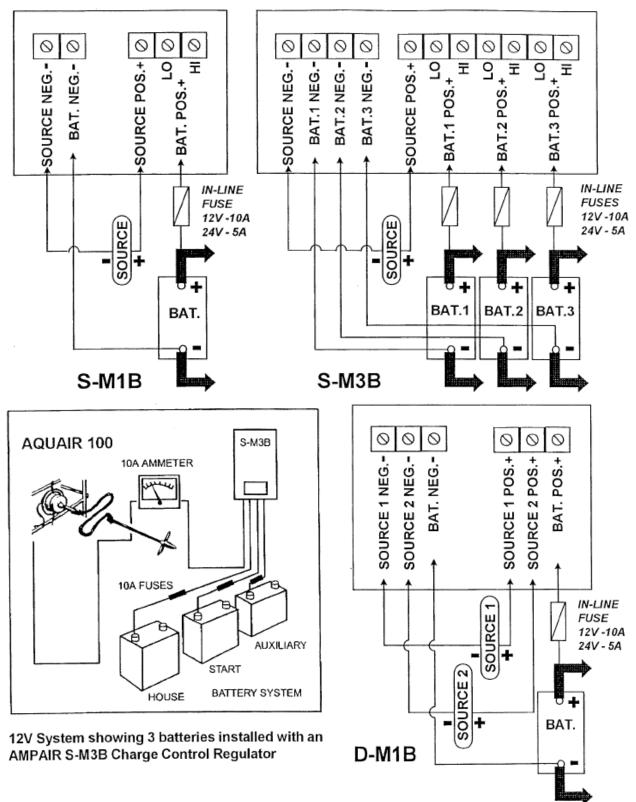
Figure 13: Charge control regulators
