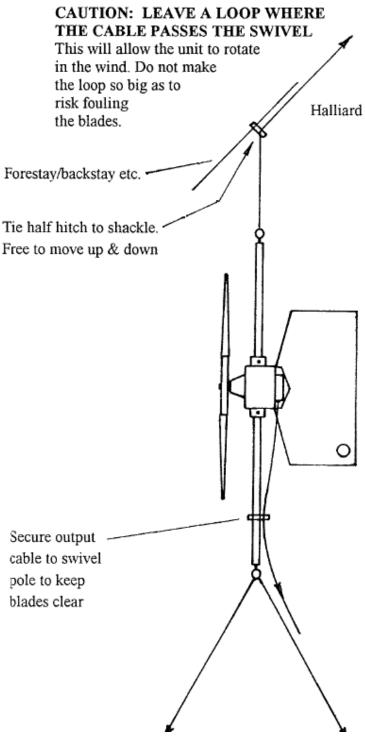
Figure 8: Aquair Hoist In Rigging Mounting
