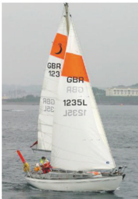
'Safety orange' stands out well in a grey sea or sky. Here Bill Hockley has added some orange storm canvas to the sails of his Cutlass 27. This bright sailcloth also provides extra reinforcement when the main is heavily reefed
