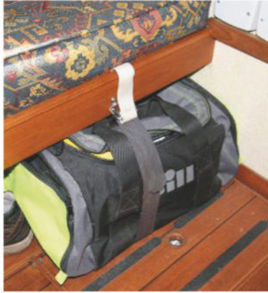
Everything secure. This stowage bag has been physically attached to the bunk via a strap. Note the screws in the floorboards. Non-essential access boards are secured, and hatches over seacocks are fitted with turnbuckles for quick inspection
