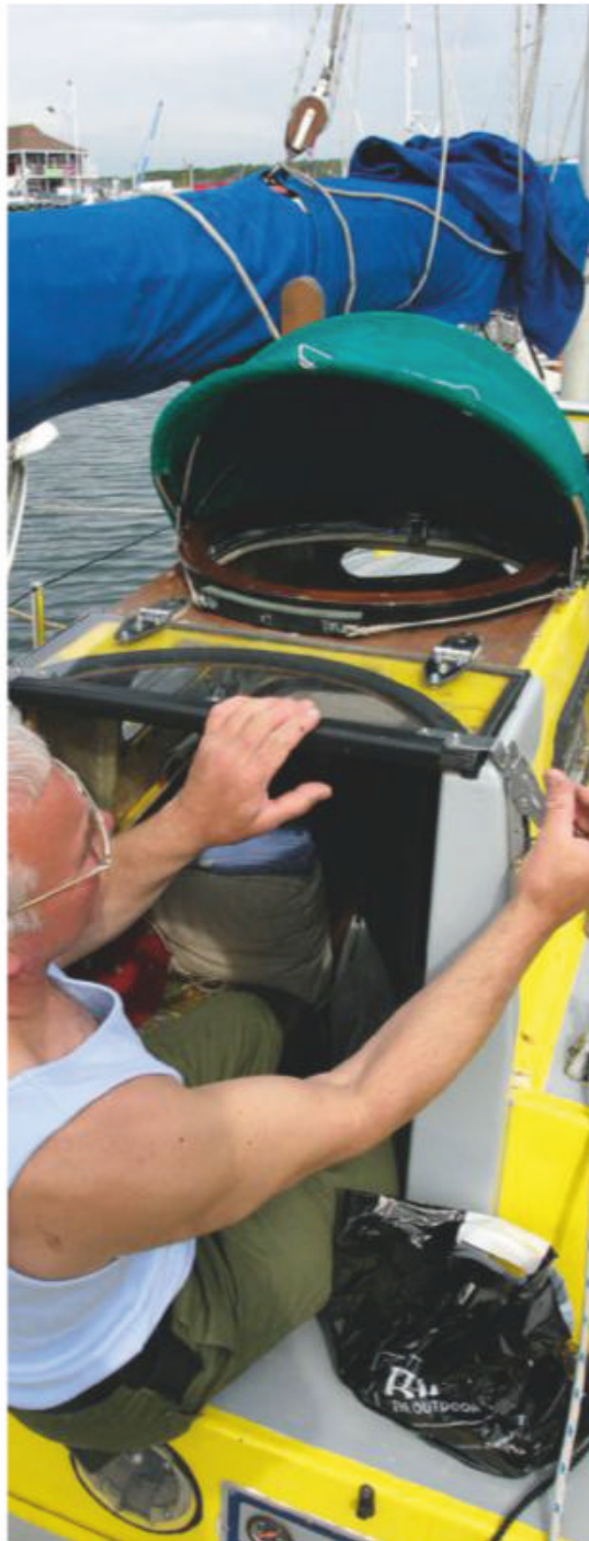
Graham Jewitt removed the original main hatch on his Kingfisher 22 and built a pilothouse over the void. This gave him full standing headroom. Note the rotating pram hood for a circular lookout hatch
