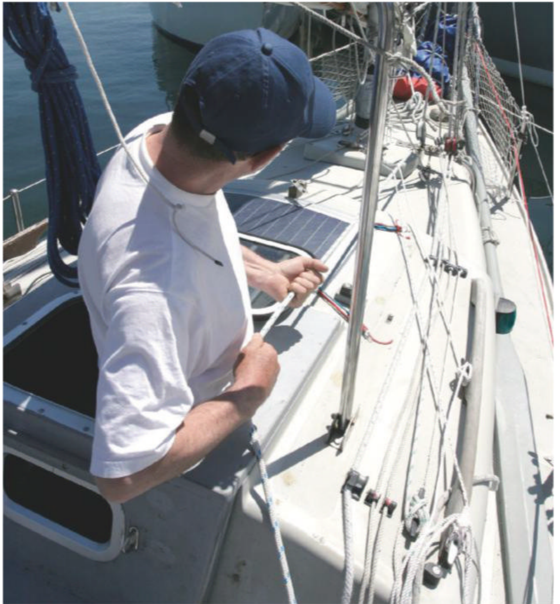
Junk rig is remarkably easy to use from the safety of the cockpit. Here Roger Taylor demonstrates how Mingming's halyards are operated without ever going on deck. He later took this 21ft engineless Corribee deep into the Arctic. (See 'Voyages of a Simple Sailor' review on p40)
