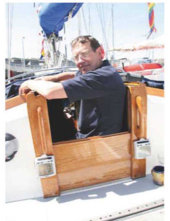
Duncan Lougee built a watchkeeping seat for his Rustler 31. It drops into slots at the top of the companionway and allows him to sit in the main hatch. The sprayhood offers good forward protection in a head sea
