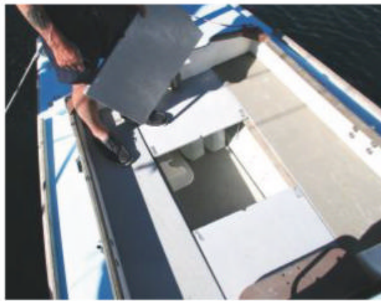
Placing boards over the cockpit not only minimises the volume of shipped water, it also gives extra stowage – and a nice place to sunbathe
