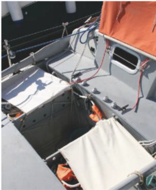
Roger Taylor filled his cockpit with his series storm drogue, which is pre-attached to strongpoints on each quarter. To deploy, he reaches out from the hatch, pulls open the white canvas covers and feeds the drogue overboard. Note the bridge deck and sealed-up companionway to reduce volume
