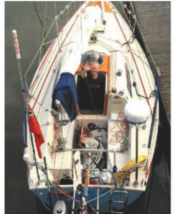
Scanning radar is relatively rare in a Jester fleet, but some small yachts still carry it. Ron Wescott's Hunter Sonata 23 is seen packing a scanner and an 'active' radar target enhancer. With power generation limited, radar tends to be used only when in fog or crossing shipping lanes
