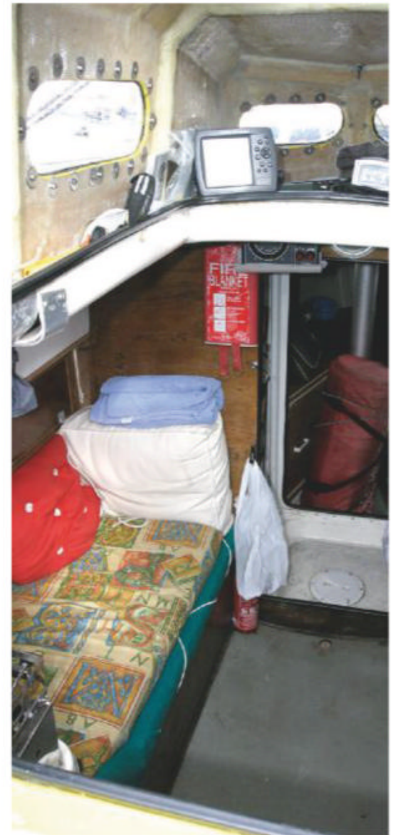
Golden Dragon's bunking arrangements under its new pilothouse. Note the rolled-up green lee-cloth, the white waterproof bag to keep the sleeping bag dry and the good visibility from the standing position. The old hatch edge acts as a hand-hold
