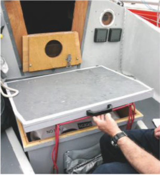
Prime Suspect's Bill Hockley has placed his liferaft container right by the (modified) hatch of his Cutlass 27. It's in the right place for an emergency and its size halves the volume of the cockpit, giving the drains a fighting chance if swamped
