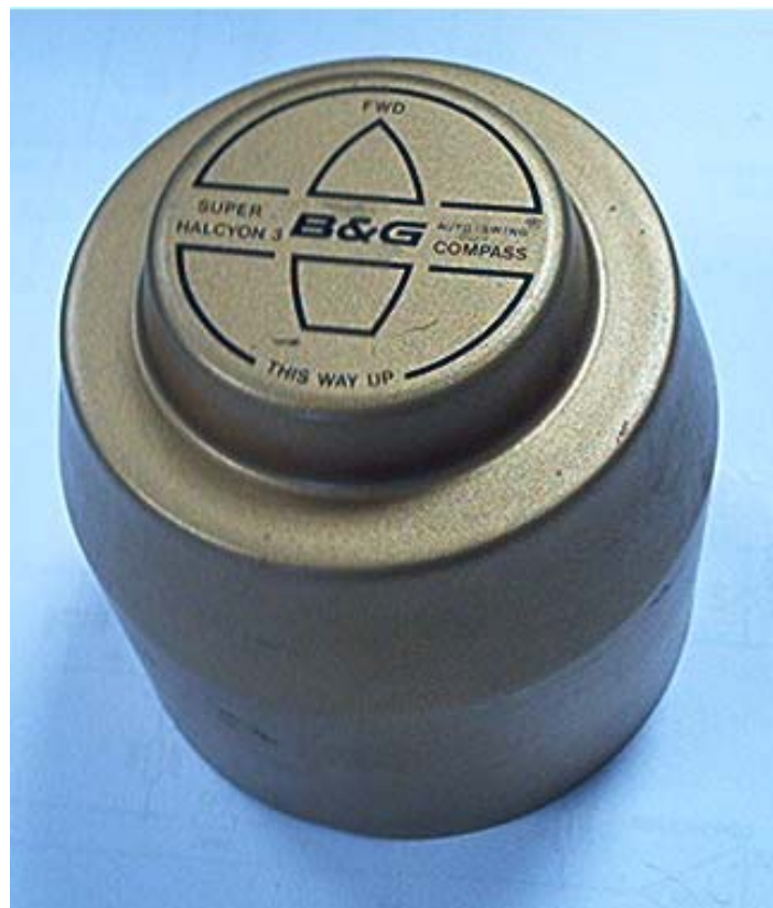
Sensor viewed from the top showing mounting orientation (Later models were white in colour)
