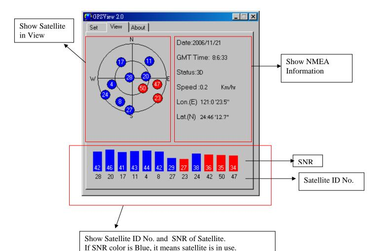
If SNR color is Red, it means satellite is under tracking. If SNR color is Gray, it means satellite is been searching.
