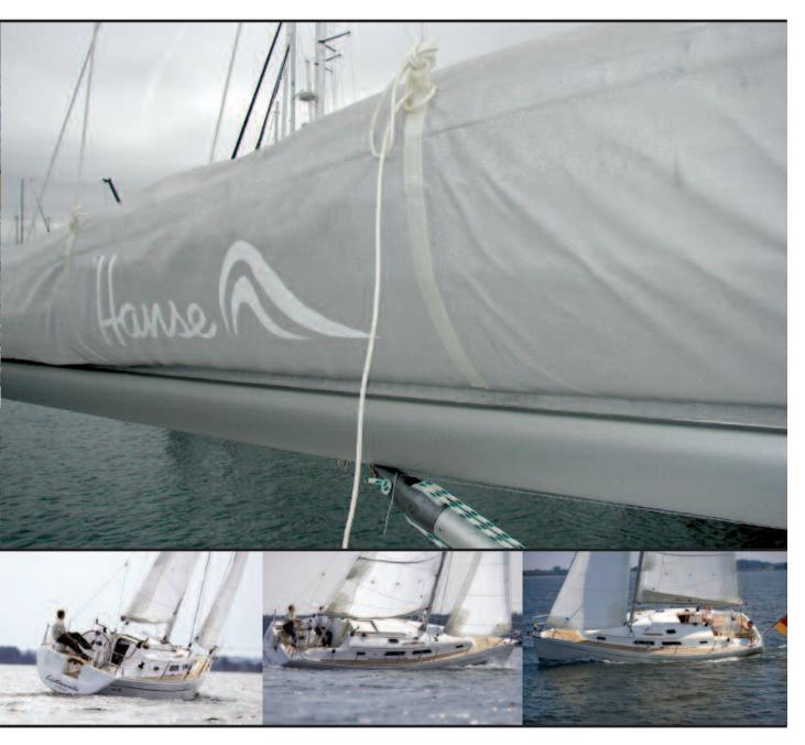
attention to the little things sets this boat apart. A clean deck layout leads the control lines aft and the self-tacker is such a nice touch making this boat a dream to sail alone or with family and friends. On the bow there is a large anchor locker and well designed bow fitting with integrated socket for a gennaker pole. Neat touches everywhere you look.
