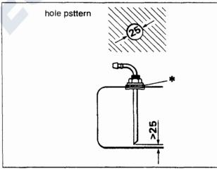
\* tank extracting device only to be used with metal fuel tanks
