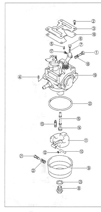
1 Idle adjusting screw (1) 2 Screw (4) 3 Plate (1) 4 Main air jet (1)
