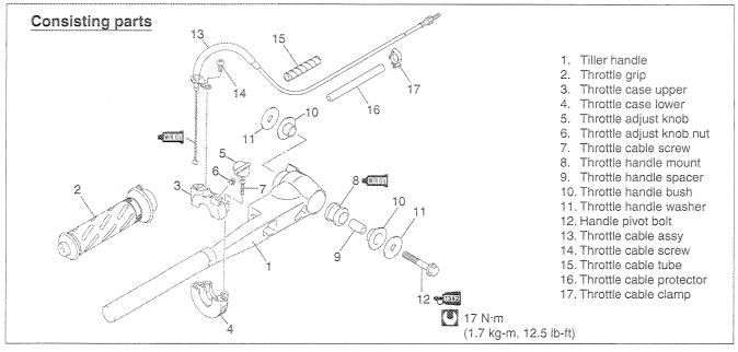
• Apply the Water Resistant Grease to the throttle handle mount ①.
