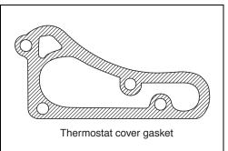
3. Install the gasket (2) and the thermostat cover (3) to the cylinder block and secure with the two bolts ④.
