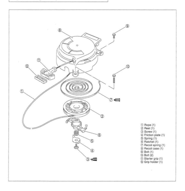
1. Turn the reel ① clockwise in order to release the coiled tension in the recoil spring.
