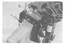
Remove the tilt lock bolt 2 and the thrust block with the lower thrust mount 1.
