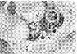
7. Make sure the retainers are properly seated in groove B.
