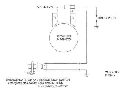
Engine stop switch: Button pushed→STOP
