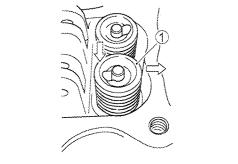
2. Remove the valve springs 2.
