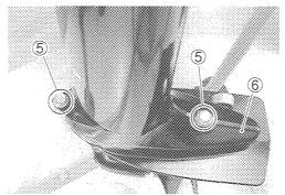
7. Remove the gear oil drain plug (8) before the gear oil level plug  $\mathcal{T}$  and drain the gear oil.
