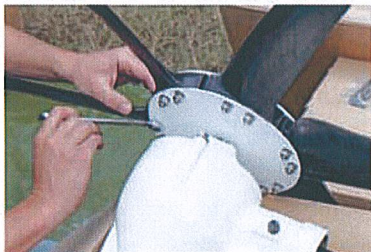
The blades were fixed at a pre-set angle in a clamping disc
