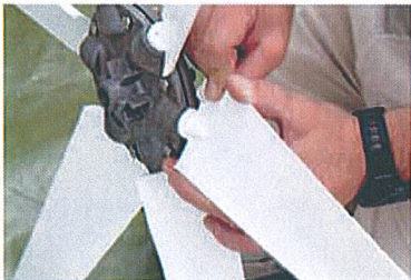
During assembly, setting the angle of the blades was a rather fiddly procedure
