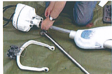
The alternator is driven by an air turbine, or water impeller
