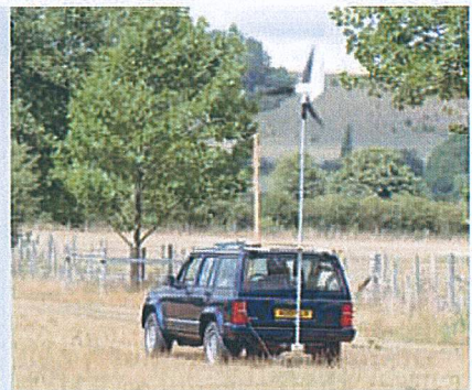
The turbines were mounted 2m above the roof to reduce turbulence as we drove upwind
