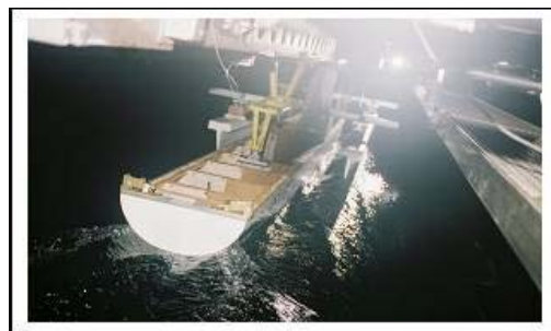
Figure 7. Center Hull @ 11.5 m Draft. Side Hulls in Fwd Longitudinal & Inboard Transverse Location @ 7.5 m Draft - 35 Kns
