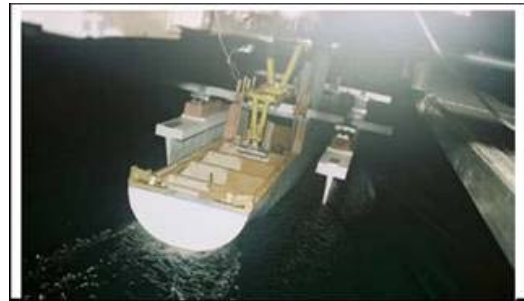
Figure 6: Center Hull @ 11.5 m Draft. Side Hulls in Middle Longitudinal & Inboard Transverse Location @ 7.5 m Draft 35 Kns
