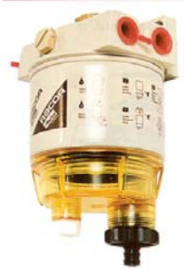
F.320R-RAC-01 FILRE GAZOIL 227 l / h bol transparent. Cartouche de recharge 10µ F.3213
