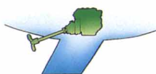
MS2B-R (R-reverse gear) Propeller shaft, 7 degree angle
