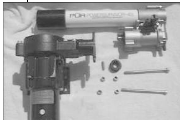
Figure B-2: Pump separated from drive assembly
