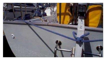
The steering lines leading forward. Looking up the port side of the boat, you can see the steering line leading from the rudder to a block on the transom, then forward to a winch. The attachment of the line to the head of the rudder is too loose, and will not work correctly as it is shown here. A tighter knot, which will eliminate slippage of the line would be a big improvement.
