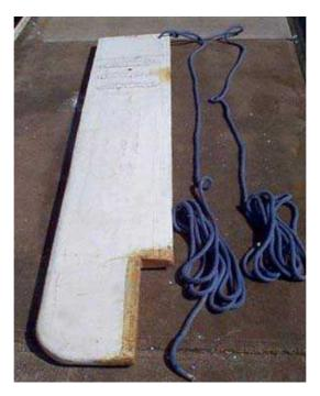
Well, it is an EMERGENCY rudder! This is a view of the emergency rudder viewed from the bottom of the "blade." The notch was installed to allow the rudder to fit a storage position on the boat. Notice that the blade is not terribly refined, and that is ok. There is only so much time you can spend on something which hopefully you will never use!
