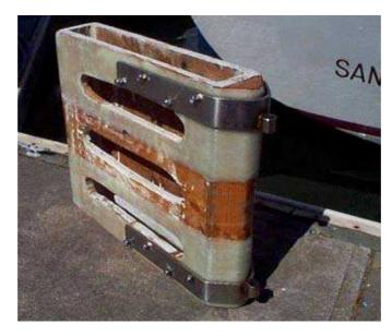
The cassette into which you slide the emergency rudder. The cassette is simply a plywood box, open on the top and bottom, "ported" for lightness(!), and reinforced with fiberglass. The rudder blade itself will slip though the cassette from the top to the bottom, then be pinned in place.
