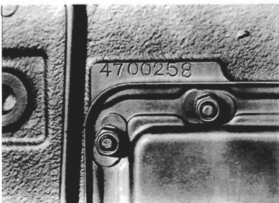
Engine Number Location (4.236 Phase I Type)
